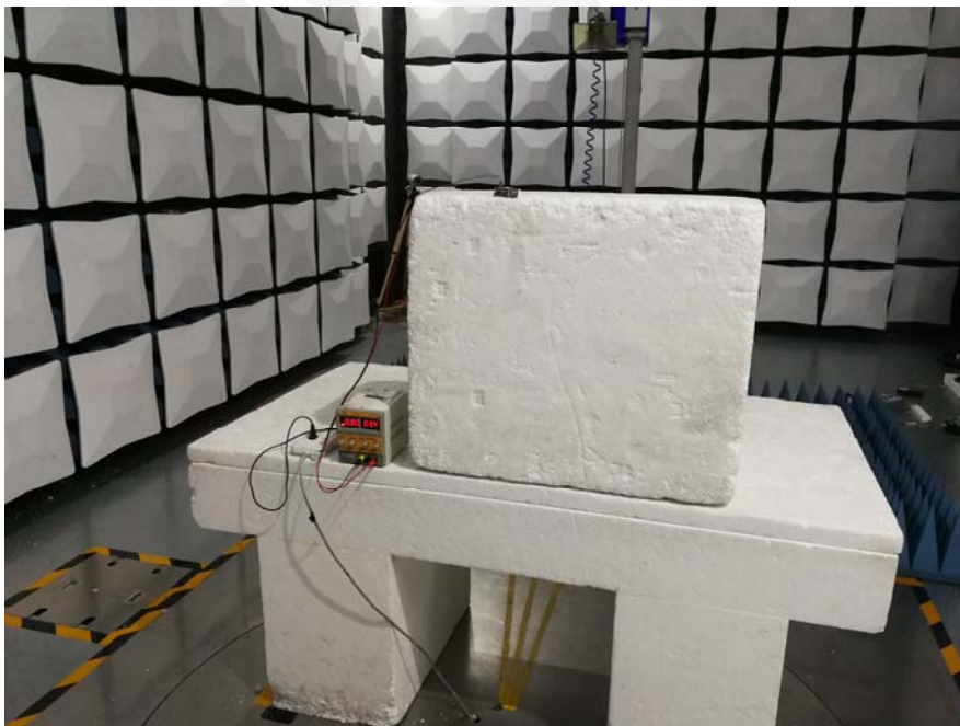
Radiated Spurious Emissions Test View (Above 1GHz)
